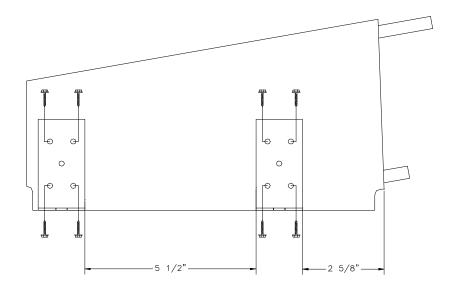
2) Use soldering iron, if necessary, to melt holes in open strap, as shown.
