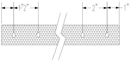
3) Use soldering iron, if necessary, to melt holes in closed strap, as shown.
